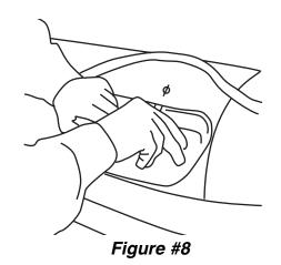
**Step 10 -** Attach the pad to the inflatable, see figure #8, and rub the air out from under the pad using a hard roller or rounded stick. See figure #9. You may want to deflate the boat to assure a better bond for the pad. It is critical to get all the air out from between the pad and the inflatable and the pad is sealed around the edges.
