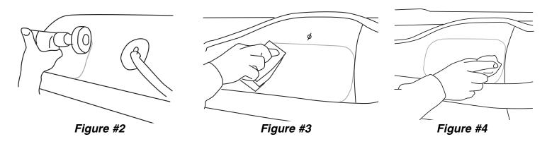
**Step 5 - (ONLY FOR HYPALON BOATS)** Once you have the proper glue you will need to sand the surface of the inflatable where the pads are to be glued. You can do this by using a sandpaper floppy disc you attach to a drill motor or by hand with 60 grit paper. **Be very careful not to damage boat.** The surface of the inflatable should now be cleaned with the proper cleaner to remove any trace of finger oils or dust. See figures #2, 3, and 4.
