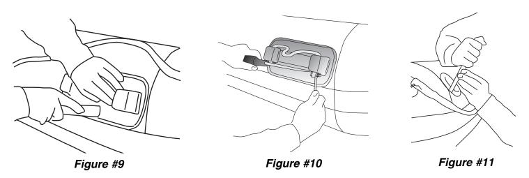
**Step 11 -** Once the air is out from under the pad, let the pad set-up for 48 hours. \*\***DO NOT TOUCH IT!!**\*\* After 48 hours attach the stainless steel yoke with the 3/4" long hex head bolts. A little grease on the bolt will keep the threads from gauling. The glue will be 100% set in 7 days. See figure #10.
